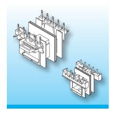
The coilformers are fitted with solder-pins and solder-tags. By fitting shrouds and insulating bridges creepage- and clearance distances of 11 mm/0.433 inch are achieved between primary and secondary, and 6 mm/0.236 inch to the core.
