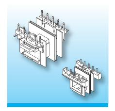
The coilformers are fitted with solder-pins and solder-tags. By fitting shrouds and insulating bridges creepage- and clearance distances of 11 mm/0.433 inch are achieved between primary and secondary, and 6 mm/0.236 inch to the core.
