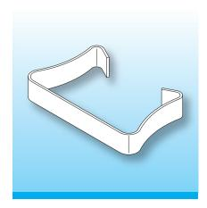
One clip is required to assemble a wound coilformer with one pair of ferrite cores. The use of a drop of glue is recommended, to connect the ferrites to the coilformer and to prevent frequency noise. Dimensions in mm/inch.
