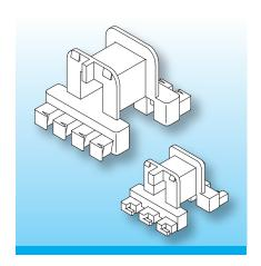
The coilformers have no metal terminals. Wires are connected to plastic feet, which have a v-shaped slot for wrapping. The binding-on points of the wires provide the eventual connection to the pcb. These soldering points should be brushed blank before positioning onto the pcb.
