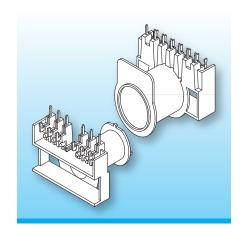
The ETD safety class coilformers have the advantage that the primary and secondary windings are wound separately on the coilformer halves, with the two windings pushed together to form a complete winding assembly.
